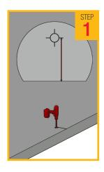
Drill 1no. ØM12mm/½" x 85mm/3½" deep hole 100mm/4" in from edge to accept a øM12mm/½" x 75mm/3" Thunderbolt or equivalent to manufacturer's specification.
