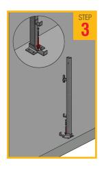
Screw 1no. ØM12mm /½" x 75mm/ 3 " Thunderbolt or equivalent into holes and ensure it is tight.
